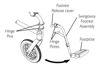
FIGURE 6.1 Installing/Removing/Using the Footrest/Legrest
